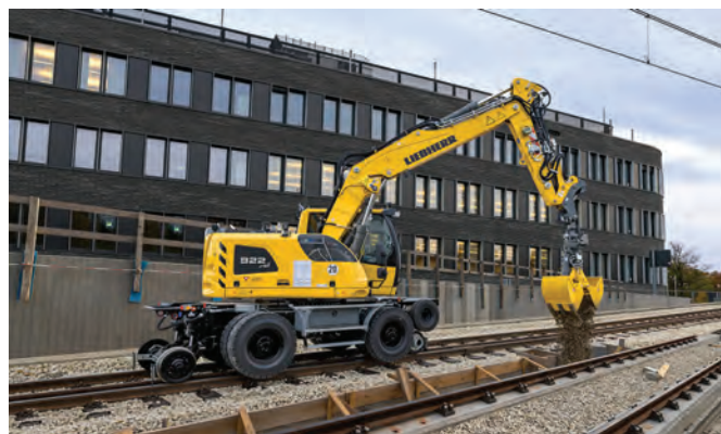
FROM TOP: Liebherr's LB 45 drilling rig, HS 8200 duty cycle crawler crane, and A 922 Rail Litronic rail-road excavator.
