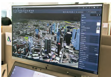
Autodesk’s virtual model of Singapore with a wide pool of data allows users to not only explore and conceptualise their infrastructure projects, but also optimise their designs by using flood simulation and dynamic site analysis.
