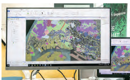
Bentley Systems’ open and federated workflows enable data sources from various agencies to be integrated, while keeping it in its native file format. The above image shows data from CityGML, GeoTIFF, Shape and DEM files.
