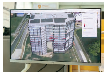
The visibility study conducted on this 3D-rendered building on the ArcGIS platform, from Esri Singapore, allows users to identify the clearest line of sight at each level, gauged by the distance of the furthest visible point.
